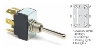
Up: Park, Tail & Headlamps - Center: Off - Down: Park, Tail & Auxiliary Lamps. Six blade terminals. Long handle.
