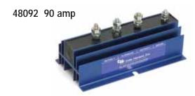
Terminations: three 1/4" (6.4mm) studs and one No. 10 stud. Two 9/32" (7.2mm) diameter mounting holes. Size: 6 1/2"L x 3 1/4"W x 2 13/16"H (165.0 x 82.6 x 71.0mm).
