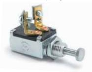
7/16" -20 thread mounting stem, 7/16" long (11.1mm), two flats on stem for mounting in double-D hole. Two screw terminals, plated steel case. 10A at 12V DC.
