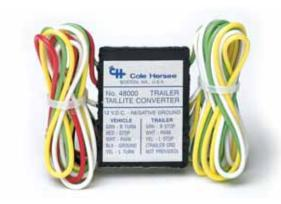
Permits a towing vehicle with two lighting circuits for each side to operate lights on a trailer with a single circuit each side. Eliminates the need to rewire the trailer, or to add additional lights. US laws require stoplights, turn signals and taillights on trailers.
