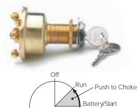
Key removable in Off position, spring return to RUN. Electrical ratings at 12V DC: 2A Magneto, 10A Battery/Ignition, 3A Choke, 5A Start.
