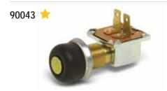
20A at 12V DC, 10A at 24V DC. Silver contacts. Rubber cap snaps into special groove and is secured to the mounting stem by a deep-threaded nut for a positive seal. Two blade terminals mate with two-pole Delphi (Packard) connector 2977647 or equivalent. 5/8" -32 thread mounting stem, .625" (15.9mm) long. Gasket-sealed case. Steel plunger protrudes through the cap.
