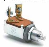
10A at 12V DC. Normally Off. Pull On, spring return to Off. Brass case and mounting hardware. Two screw terminals with lockwashers. Mounting stem 1/2"-20 thread, 5/8"(15.9mm) long. No knob: shaft has 3/32" (2.4mm) hole for the attachment of a cable or lever.
