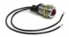
12V #53 bulb supplied. 17/32" (13.5mm) diameter lens. 3/4" (19.1mm) diameter mounting stem, 11/16" (17.5mm) long. Chrome-plated brass bezel, 7/8" (22.2) diameter. Available with custom imprinting: contact Cole Hersee.
