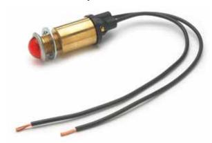
Red lens, 5/8" (15.9mm) diameter with honeycomb pattern on the internal side. Satin finish stainless steel bezel, 3/4" (19.1mm) diameter. 1/2" (12.7mm) diameter mounting stem. 7/8" (22.2mm) long. 12V #53 bulb supplied.
