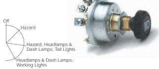
With black knob imprinted with SAE headlamp symbol. Silver contacts. Five screw terminals. Plated steel case. Mounting stem 5/8"-32 thread. With O-ring seal in the mounting stem. 20A per circuit at 12V DC.
