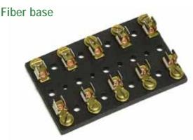
Nickel-plated phosphor-bronze plated fuse clips. Hard fiber insulator base with 11/64" (4.4mm) diameter mounting holes. Width: 2 1/4" (57.2mm), height 5/8" (15.9mm). Plated steel terminals and screws or (with M- prefix numbers) with brass terminals and screws. Mounting holes .75" (19.0mm) on centers.
