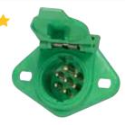
Color-fast green glass-filled plastic insures guick identification. Spring-loaded door is marked 'Trailer ABS' to further lessen any chance of misconnection. Mounting holes on the flanges are oval, .488" x .328" (12.4 x 8.3mm), 2.93" (74.6mm) on centers. Mounts through 2" (50.8mm) diameter hole.
