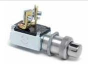
15A resistive, 10A inductive at 12V DC, 8A resistive, 5A inductive at 24V DC. Two screw terminals. Mounting stem: 5/8"-32 thread, .87" (22.1mm) long.
