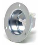
Faceplate only: does not include switch. Needs to be countersunk in a 2" (50.8mm) hole. 3 3/16" (81.0mm) diameter with three 7/32" (5.6mm) holes on a 2 3/4" (69.9mm) diameter circle. Requires a clearance depth of .890" (22.6mm), not including clearance for a switch. Other colors, metals and finishes are available on special order. Contact Cole Hersee.
