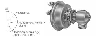
With short diecast lever. Four screw terminals. Plated steel case. Mounting stem 5/8"-32 thread. With O-ring seal in the mounting stem. 20A per circuit at 12V DC.
