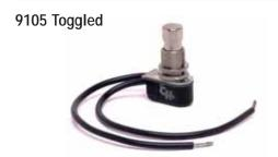
10A at 12V, 5A at 24V. Two 6" (152.4mm) wire leads, 16AWG (1.00mm<sup>2</sup>). Phenolic body, 1.080"L x .530"W x 1.10"H (27.4 x 13.5 x 28.0mm). Push-button diameter .410" (10.4mm). Stem: .470" long (11.9mm). Can be used as a foot switch in dry environments.
