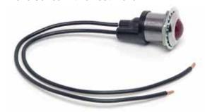
17/32" (13.5mm) diameter lens. Chrome-plated brass bezel, 7/8" (22.2mm) diameter. 3/4" (19.1mm) diameter mounting stem, 1 1/16" (27.0mm) long. 12V #53 bulb supplied. Available with custom imprinting: contact Cole Hersee.
