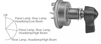
With black nickel-plated lever actuator. Five blade terminals, accepts Delphi (Packard) connector 2962912. Plated steel case. Mounting stem 5/8"-32 thread. With O-ring seal in the mounting stem. 20A per circuit at 12V DC.
