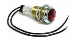
Insulated. 12V #68 bulb supplied. 15/16" (23.8mm) diameter faceted lens, gasket-sealed. 7/8" (22.2mm) diameter mounting stem, 3/4" (19.1mm) long. Plated brass bezel, 1 1/4" (31.8mm) diameter.
