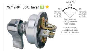
Heavy duty 50A switch allows forward and reverse motion of a motor without the need for a relay, especially for operation of tarps on trucks. Heavy duty component parts: 3/32" thick terminals, silver-laminated contacts to resist arcing over a long working life. 2.09" diameter (53.1mm) steel case. 10-32 x .375" (9.5mm) terminal screws with lockwashers. Mounting stem 1/2" -20 thread.
