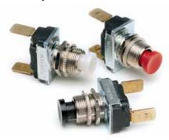
5A at 12V to 24V DC. Two blade terminals .250" wide (6.4mm). Nickel-plated brass hexnut and facenut. Nylon push-button, .410" diameter (10.4mm). Body size (to top of terminal): .890"L x .560"W x .773"H (22.6 x 14.2 x 19.6mm).
