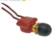
PVC-coated body sealed against moisture and dirt, with black rubber snap-on cap 407-03. Two 12" (304.8mm) 18AWG leads. Brass mounting stem 5/8"-32, 15/16" (23.8mm), fits panels up to 1/2" (12.7mm) thick.
