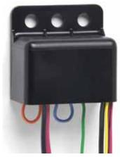
Wiring: 2 power in, 2 power out, control wire to momentary switch. Instructions are included. Power wires 16AWG control wires 18AWG, loops 22AWG. System voltage 12V DC (9-16V).
