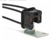
Accepts standard 3-prong flasher units (not included). Molded plastic connector has 14AWG wire leads, with phosphor-bronze contacts. Comes with plated steel bracket that has two .203" (5.2mm) diameter mounting holes.
