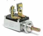
7/16" -20 thread mounting stem, 7/16" long (11.1mm), two flats on stem for mounting in double-D hole. Two screw terminals, plated steel case. 10A at 12V DC.
