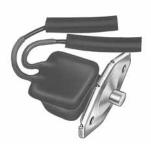
15A at 12V DC. With special diaphragm/mounting bracket, sealed to protect the mounting shaft. Plasticized body protects against moisture and dirt. Two 16AWG wire leads, 3" (76.2mm) long with female bullet terminals. Insulator sleeves protect the connections. 13/64" (5.2mm) diameter mounting holes, 1 1/2" (38.1mm) on centers. 1/4" (6.4mm) long plunger.
