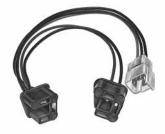
For Chevrolet and GMC RVs. Accepts one 3-prong headlamp and one 2-prong headlamp. This harness attaches to a 3-pole Packard connector that is supplied with the vehicle chassis. Leads are 16AWG wire that connects into silvered bronze contacts in molded plastic connectors.
