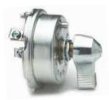
Lever actuator and indexing pin. Four screw terminals. Plated steel case. Mounting stem 1/2"-20 thread. With O-ring seal in the mounting stem. Silver contacts. 30A total at 12V DC.
