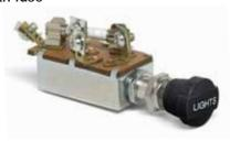
With 20A at 12V glass fuse, black knob imprinted 'Lights'. Four screw terminals, plated steel case, mounting stem with 7/16"-28 thread.
