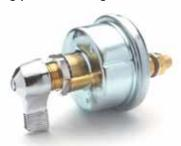
Diecast lever. Plated steel case. Silver-laminated contacts. Brass mounting stem 3/4" -16 thread 17/32" (13.5mm) long. Fits panels through 1/4" (6.4mm) thick. Two 3/8" -24 and two 10-32 studs. O-ring seal in the operating shaft, and gasketsealed terminal insulator.
