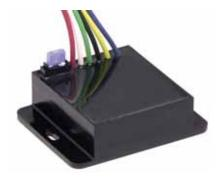
Automatically turns on low-beam headlights when the ignition is turned on (after a 10 second delay, thus reducing the initial starting load. Activated when the parking brake is released; deactivated when the parking brake is set (with ignition On). Deactivates when high beams are flashed for signaling. Completely solid-state construction. Supplied with 15A minifuse ATM98107-15.
