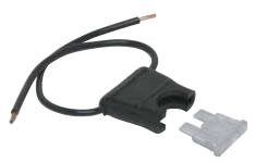
Accepts ATO and ATC fuses and circuit breakers from 3A to 20A. Easy to install and easy to change the fuse. 16AWG insulated copper wire leads, 4" (101.6mm) long. Brass contacts. Supplied without a fuse.
