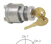
Key removable in both positions. Electrical ratings at 12V DC: 10A both positions. Three brass screw terminals. Diecast case. Mounting stem 3/4" -20, 13/16" (20.6mm) long, fits panels up to 1/4" (6.4mm). Knurled aluminum adapter facenut permits mounting in 3/4" (19.1mm) to 7/8" (22.2mm) diameter holes.
